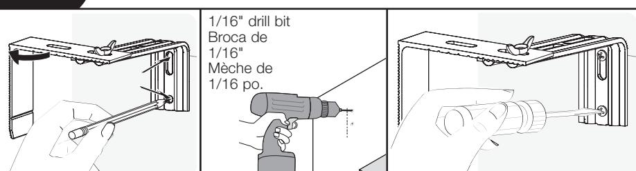
**7****Fully extend valance bracket and tighten wing nut**
